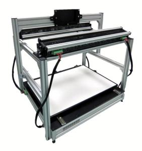
The table can be upgraded by adding the option for scanning in a second direction. This is useful if measurements with a high magnification are needed. The camera might not be able to capture the whole sample plate in one scan then, and scanning in x and y directions might be needed to cover the whole sample.
