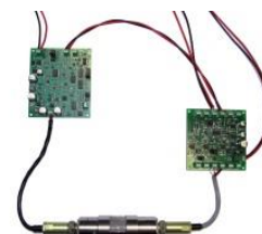
Evaluation system for CO 2 (or CH 4 ) detection
