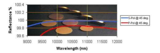
**Phase retarders** – A vacuum deposited dielectric coating that introduces a ¼ wave phase shift. This circularly polarizes a linearly polarized beam. Very sensitive to incident angle (45 degrees) and wavelength (10.6 microns). Can be made on copper or silicon.
