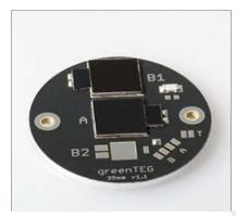
PCB-mounted Radiation Sensor
