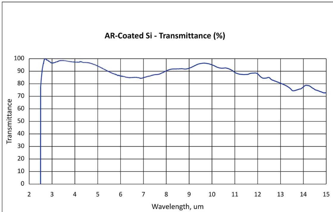
Compared to other materials AR-Coated Si is very durable and does not require special attention regarding humidity, temperature and mechanical stress.
