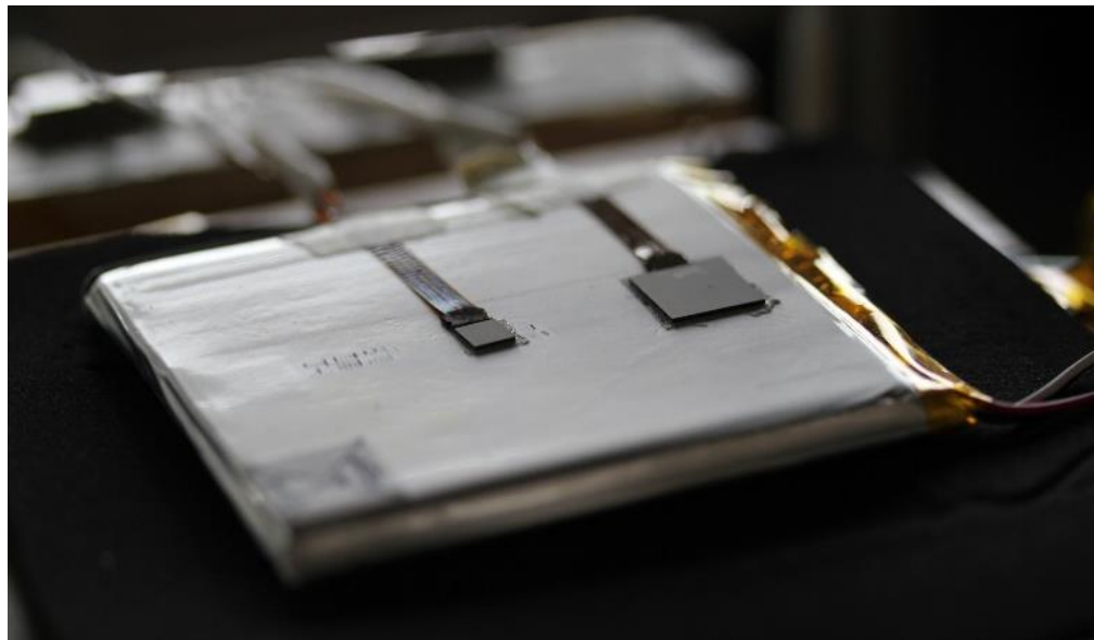
Example: Integration of gSKIN heat flux sensors into a measurement setup
