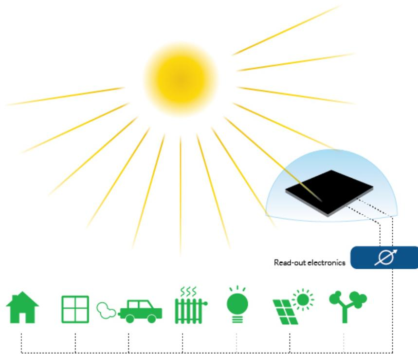
Control and trigger different applications depending on the presence/absence of sunlight. For example: heating, lighting, ventilation, and shading of buildings or vehicles, the optimal alignment of PV installations towards the sun or watering (agriculture and garden).
