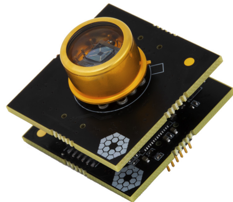
Analog component package for detector chip and TEC element
