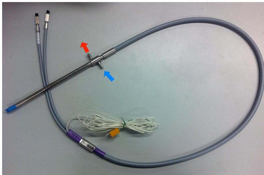
Addition for High-Temperature version of Diamond ATR probe: input and output of cooling gas should be connected as shown at the photo. The thermo junction position is approx. 12-15mm close to Diamond tip inside the shaft.
