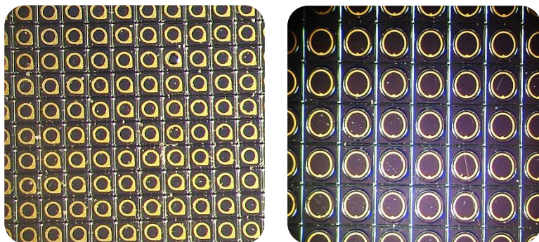
Semiconductor wafer (LED and PD chips with ring top contacts)
