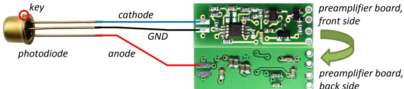
2. Solder the power supply wires: "+5V" to (3) and "GND" to (4).
