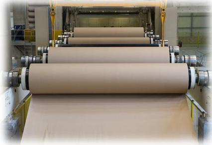
One of the key parameters of paper manufacturing is paper **moisture**. It is important to know the amount of moisture on every stage of paper manufacturing in order to control the technological process. There are several different techniques of **water** detection. We offer method of **optical absorption** based on **mid-infrared** LED-PD optopair.
