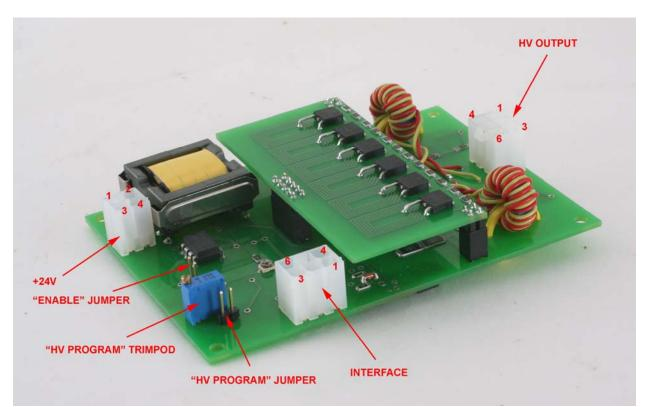
There are three connectors at Pockels cell driver board. Hereafter is description of corresponded female connectors (supplied with the board)
