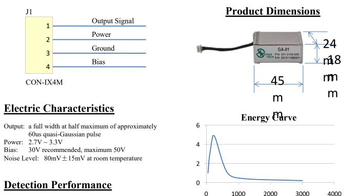
Energy Detection Range: 50keV to 3MeV Response Time: Typical 1 second Signal amplitude: 0.9V±0.1V @662keV Detection efficiency: 25000±20% count/uSv @662keV Noise Temperature Effect: Refer to PIN Diode Characteristics Working Temperature: -20°C to 50°C Life Span: 5 years
