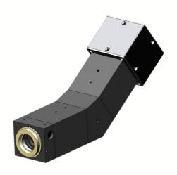
Like most inno-spec spectral imaging systems the Spectral Imaging System VNIR is based on a transmissive optical design with AR-coated lenses, a VPH grating as dispersive element and without moving parts.
