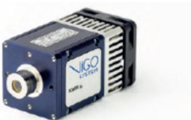
MIP is a transimpedance, AC or DC coupled preamplifier, intended to operate with either biased or non-biased detectors. It is dedicated for benchtop applications and recommended for laboratory usage. Medium-size preamplifier is a convenient device with internal built-in heat sink. MIP is integrated into package type F which is equipped with fan and does not require any additional heat sink. MIP is one of the most user-friendly preamplifiers which surely facilitate work.
