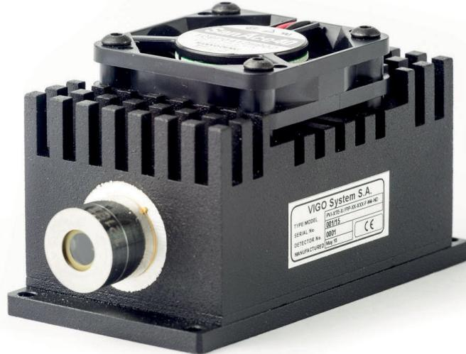
FIP is a high speed transimpedance, AC coupled preamplifier. Extremely broad bandwidth up to 1GHz guarantees quality of high speed infrared measurements. FIP preamplifier is intended to operate with either biased or non-biased TE cooled detectors. Fast preamplifier enables precise I-V conversion, detector biasing up to 800mV and simultaneously maintains compact size and keeps current noise low. FIP is suitable for laboratory usage. Additional DC output is available as an option.
