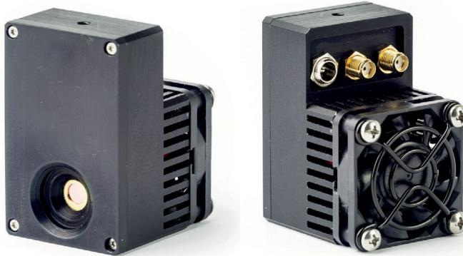
AIP is a new generation of transimpedance, AC or DC coupled preamplifier, integrated with thermoelectric cooler controller. It is designed to operate with either biased and non-biased detectors. Internal apply/voltage inverter allows to use single power supply what makes AIP very convenient in use and decreases power consumption.
