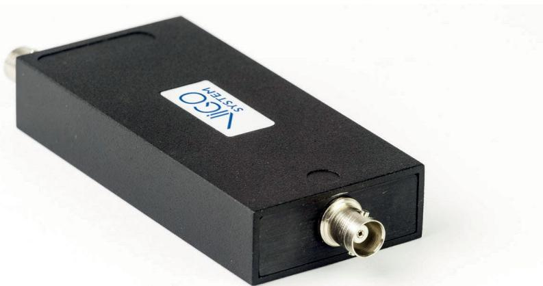
VIP is a transimpedance, AC or DC coupled, standalone preamplifier. It is intended for operating with uncooled, non-biased IR detectors in BNC packages.
