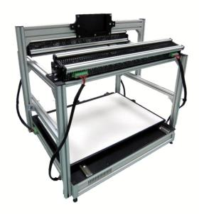
The table can be upgraded by adding the option for scanning in a second direction. This is useful with high measurements magnification are needed. The camera might not be able to capture the whole sample plate in one scan then, and scanning in x and y directions might be needed to cover the whole sample.
