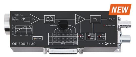
The OE-300 photoreceiver series uses premium quality photodiodes followed by a high-end, variable gain transimpedance amplifier. The low noise performance (NEP) is outstanding and the relatively large sized detectors make optical alignment easy. It has switchable gain from  $10^2$  to  $10^8$  V/A giving precise and reliable measurements within a wide dynamic range from nanowatts up to 10 milliwatts optical power.
