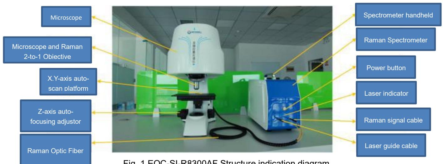
Fig. 1 EOC-SI-R8300AF Structure indication diagram
