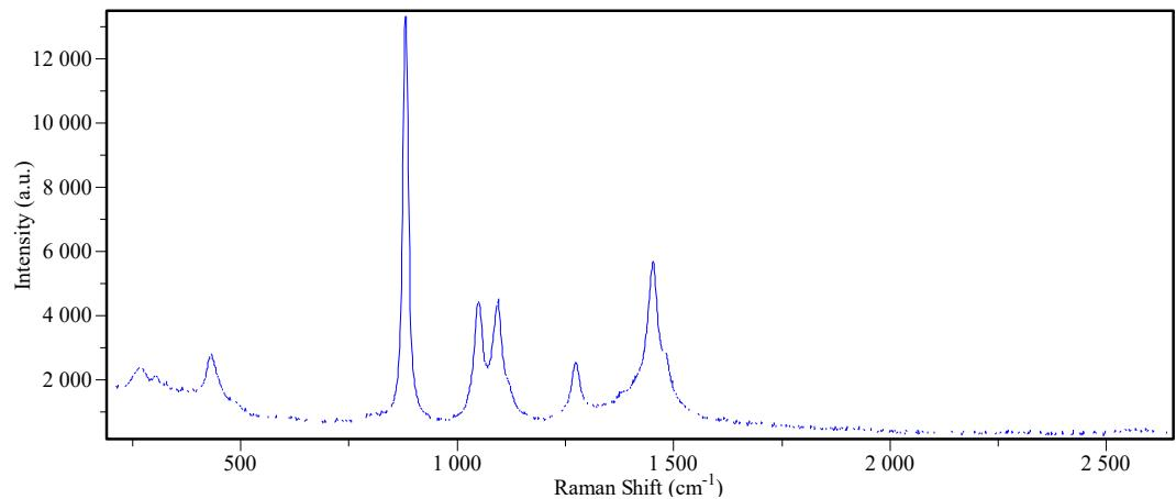
Fig 4 EOC-SI-R8300AF measure alcohol spectra (500mW, integration time:1S)
