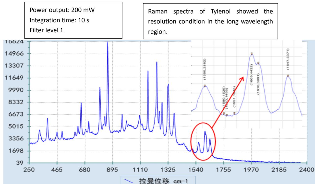
Fig 7 Tylenol spectra shows clear 1610/1615 cm<sup>-1</sup>vibration peak
