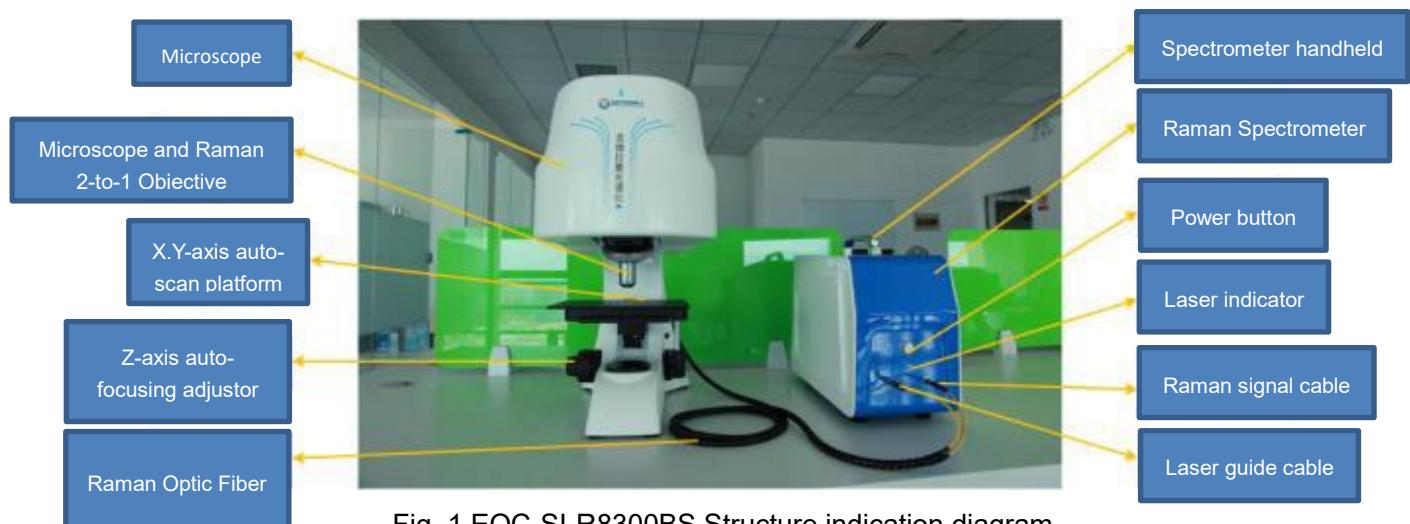
Fig. 1 EOC-SI-R8300BS Structure indication diagram
