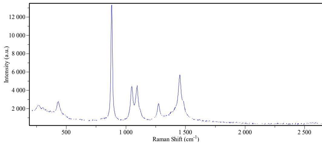
Fig 4 EOC-SI-R8300BS measure alcohol spectra (500mW, integration time:1S)
