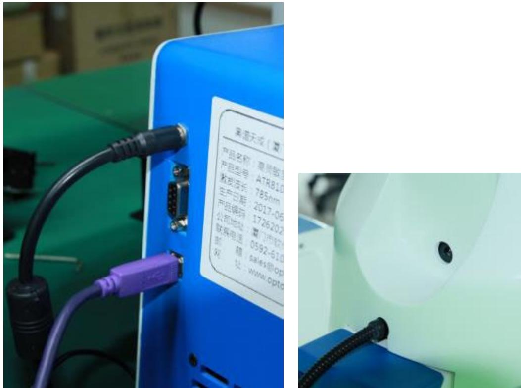
Fig 12 Simple interface: Raman microscope: power socket +USB2.0 connector
