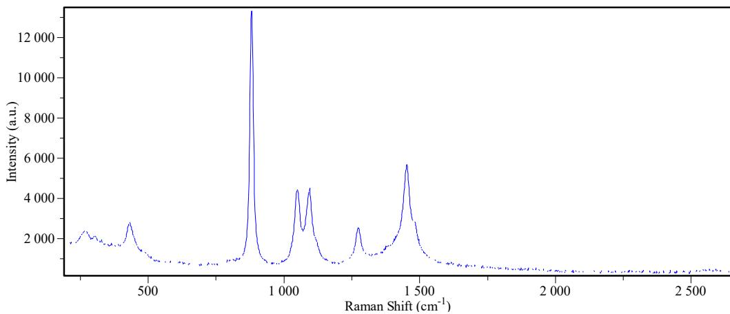
Fig 4 EOC-SI-8300 measure alcohol spectra (500mW, integration time:1S)
