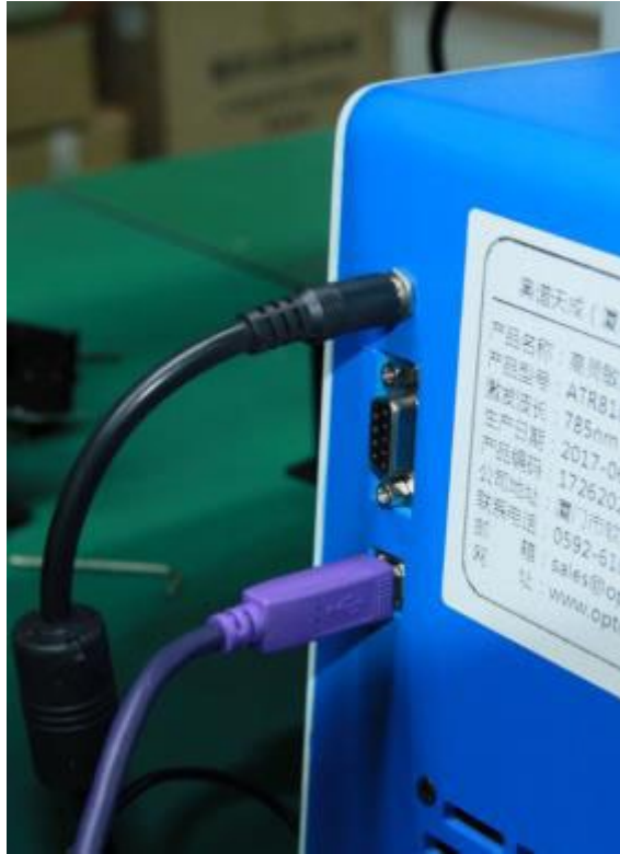
Fig 12 Simple interface: Raman microscope: power socket +USB2.0 connector
