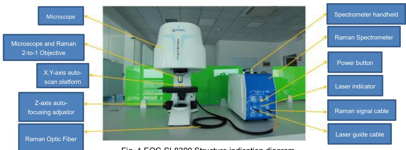
Fig. 1 EOC-SI-8300 Structure indication diagram
