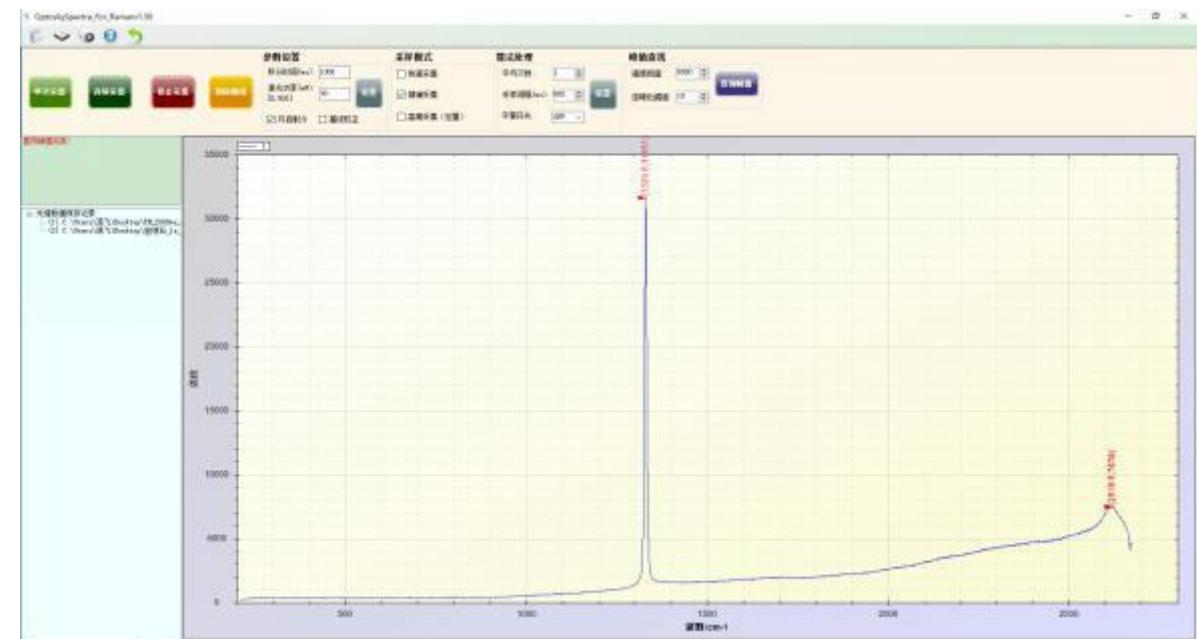
Fig 5 EOC-SI-8300 measure diamond Raman spectra (30mW, integration time: 1S)
