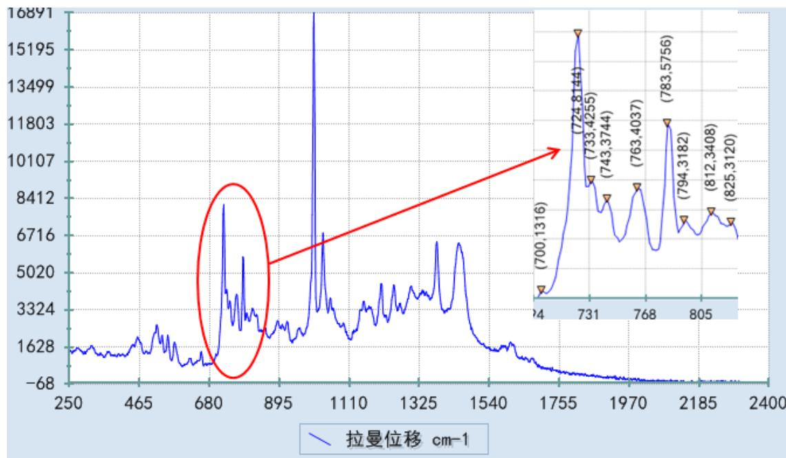
Fig 8 93# petrol Raman spectra, 723/732/742cm<sup>-1</sup> spectral shift is clearly recognized
