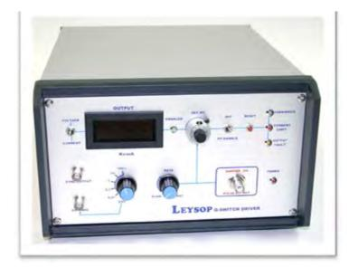
One of the most difficult aspects in dealing with electro-optic devices is the problem of working with high voltages. The majority of electro-optic devices present a capacitive load to the driver which further compounds the problem of finding a suitable driver. However, the relatively low voltage requirements of the transverse field RTP Pockels cell and similar types allow us to switch the high voltage at high repetition rates with acceptable power consumption at the driver.
