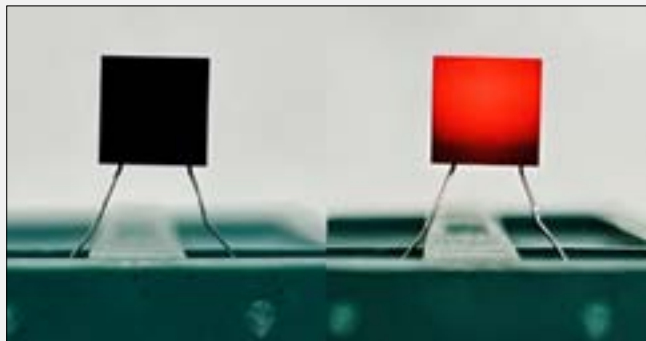
Fig. 2: Al 2 O 3 ceramic with novel black coating (left) and during operation at 1200 K (right).
