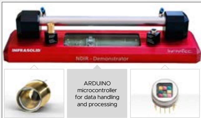
Fig. 2: NDIR-Demonstrator with HISpower series IR emitter and pyroelectric 8-channel-detector – supported by InfraTec GmbH.
